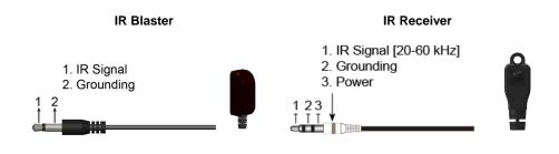
You can buy any IR extension cables in the market that are compatible to the definition of the IR sockets for the matrix if necessary for replacement use. However, IR cables longer than 2m (6-ft) may not work.
